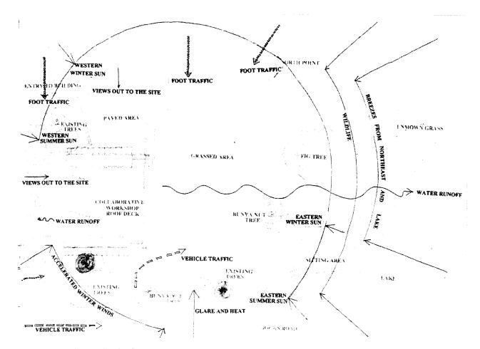
Fig. 5. Plan of energies entering the site
